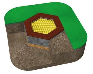
**2** The trampoline is installed in the ground at a depth of 40 cm.
